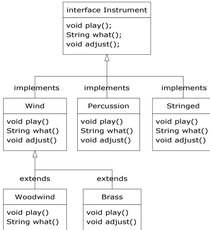
You can see from the **Woodwind** and **Brass** classes that once you've implemented an **interface**, that implementation becomes an ordinary class that can be extended in the regular way. [Feedback](#)
