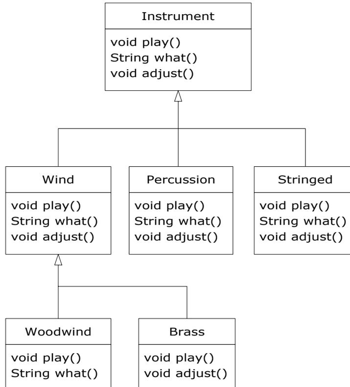
All these new classes work correctly with the old, unchanged **tune()** method. Even if **tune()** is in a separate file and new methods are added to the interface of **Instrument**, **tune()** will still work correctly, even without recompiling it. Here is the implementation of the above diagram: [Feedback](#)
