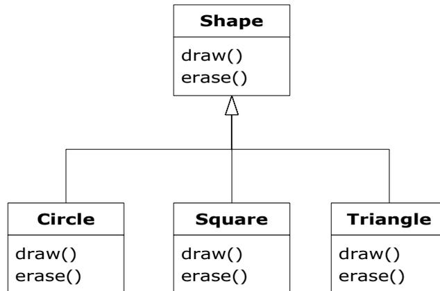
This can be called a pure “is-a” relationship because the interface of a class establishes what it is. Inheritance guarantees that any derived class will have the interface of the base class and nothing less. If you follow the above diagram, derived classes will also have *no more* than the base class interface. [Feedback](#)
