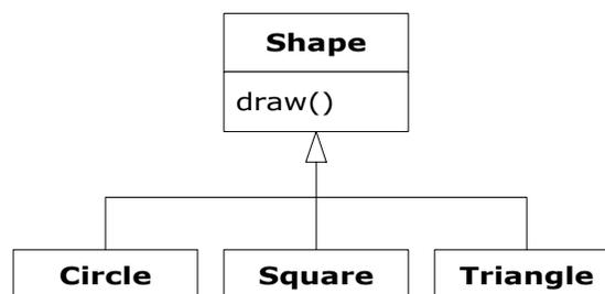
This is a typical class hierarchy diagram, with the base class at the top and the derived classes growing downward. The normal goal in object-oriented programming is for your code to manipulate references to the base type (**Shape**, in this case), so if you decide to extend the program by
