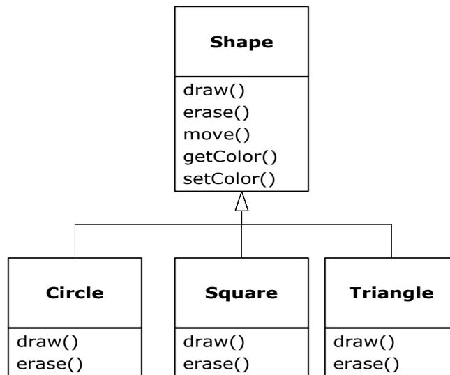
To override a method, you simply create a new definition for the method in the derived class. You're saying, "I'm using the same interface method here, but I want it to do something different for my new type." [Feedback](#)
