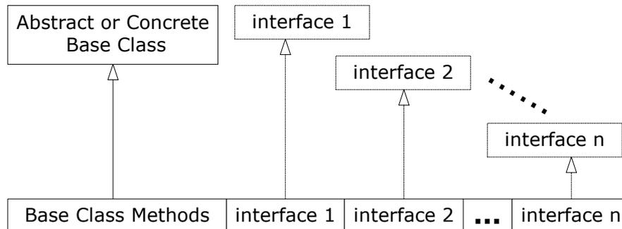
In a derived class, you aren't forced to have a base class that is either an **abstract** or "concrete" (one with no **abstract** methods). If you *do* inherit from a non-**interface**, you can inherit from only one. All the rest of the base elements must be **interfaces**. You place all the interface names after the **implements** keyword and separate them with commas. You can have as many **interfaces** as you want—each one becomes an independent type
