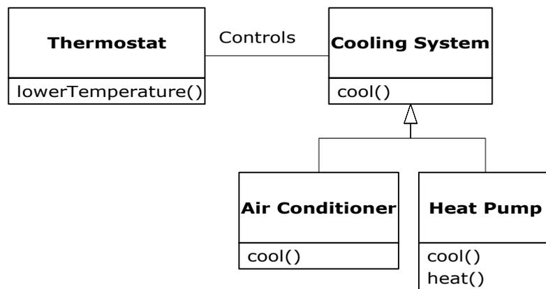
Of course, once you see this design it becomes clear that the base class “cooling system” is not general enough, and should be renamed to “temperature control system” so that it can also include heating—at which point the substitution principle will work. However, the diagram above is an example of what can happen with design in the real world. [Feedback](#)
