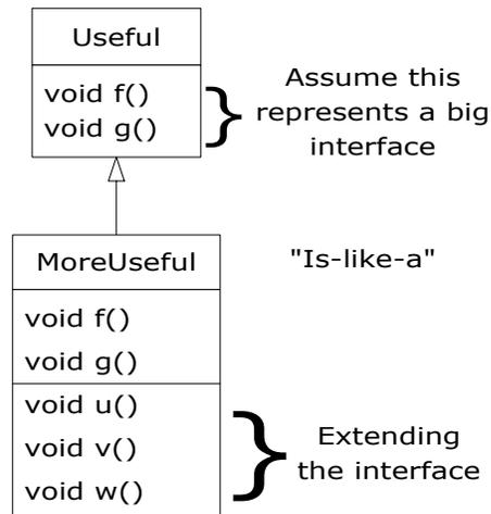
While this is also a useful and sensible approach (depending on the situation) it has a drawback. The extended part of the interface in the derived class is not available from the base class, so once you upcast you can't call the new methods:
