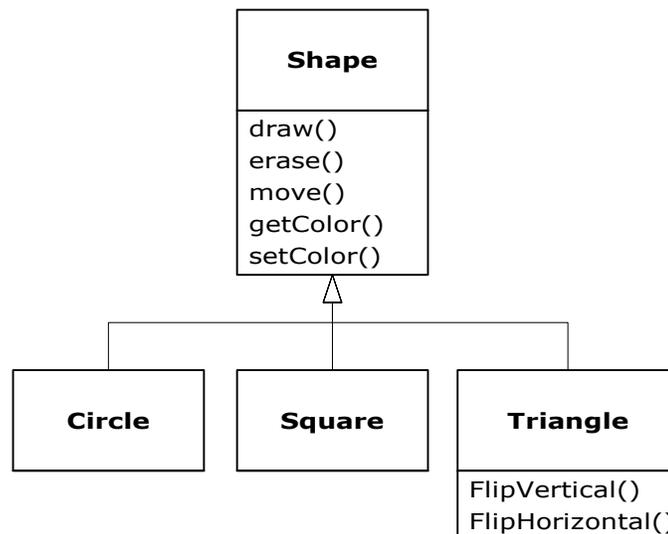
Although inheritance may sometimes imply (especially in Java, where the keyword for inheritance is **extends**) that you are going to add new methods to the interface, that's not necessarily true. The second and more important way to differentiate your new class is to *change* the behavior of an existing base-class method. This is referred to as *overriding* that method. [Feedback](#)
