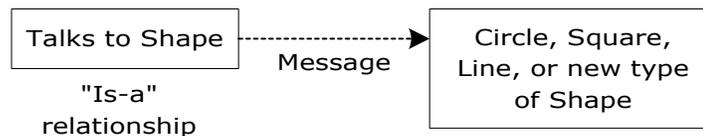
That is, the base class can receive any message you can send to the derived class because the two have exactly the same interface. All you need to do is upcast from the derived class and never look back to see what exact type of object you’re dealing with. Everything is handled through polymorphism. [Feedback](#)
